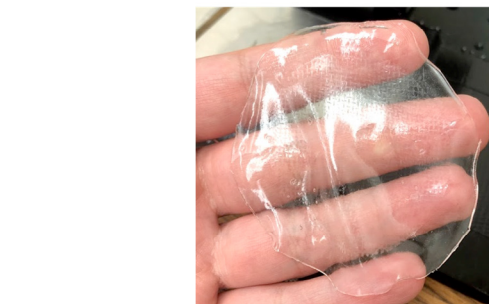
Fig. 2. (a) Process of preparation of PVC gel membrane; (b) A photograph of a fabricated PVC gel membrane.
