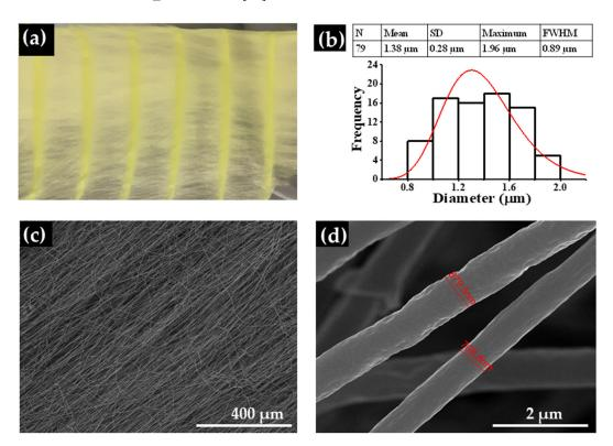
**Figure 1.** (a) Electrospun NNDM4NA@PLLA microfiber array as collected on a rotatory drum; (b) microfiber diameter distributions with average fiber diameters (mean), standard deviation (SD) and full width at half maximum (FWHM); SEM images at 250× (c) and 50,000× (d) magnification level. The fiber diameter distribution was fit to a log-normal function.
