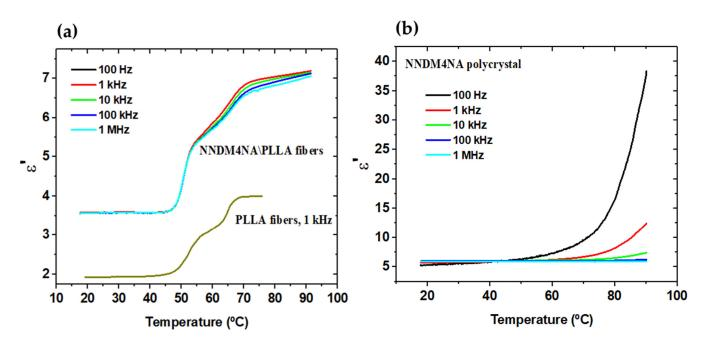
**Figure 5.** Temperature dependence of the dielectric constant (ε') at different frequencies of (**a**) NNDM4NA@PLLA and the pure PLLA nanofiber array, (**b**) the polycrystalline pellet of NNDM4NA.
