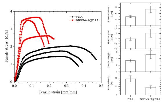
**Figure 4.** Elastic modulus, stress at yield, tensile strength and strain at break of PLLA and NNDM4NA@PLLA electrospun fibers.
