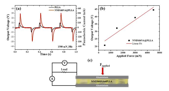
Figure 6. (a,b) Output voltage (V) and current (nA) measured through a load resistance of  $100 \text{ M}\Omega$  on the electrospun fiber array of PLLA and PLLA doped with NNDM4NA nanocrystals, (c) and schematic piezoelectric setup for the NNDM4NA@PLLA fiber array.
