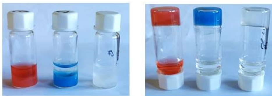
Figure 11. Representative images of hydrogels obtained from dehydridipeptide 1 loaded with MO (left), MB (centre), and ciprofloxacin (right) layered with SBF solution (1.5 mL) following a saturating release study. After 168 h, 37% of MO and 23% of ciprofloxacin were released from the hydrogel.
