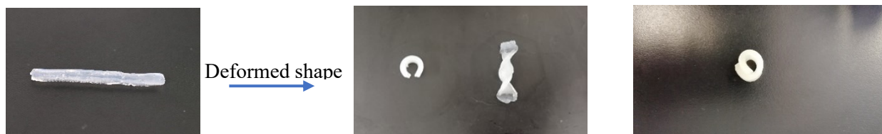
Figure 27. Photos showing the initial shape of PVA-CNC or PVA-TA hydrogel (strip), and the deformed state retained by one freezing-thawing cycle (twist, spiral).
