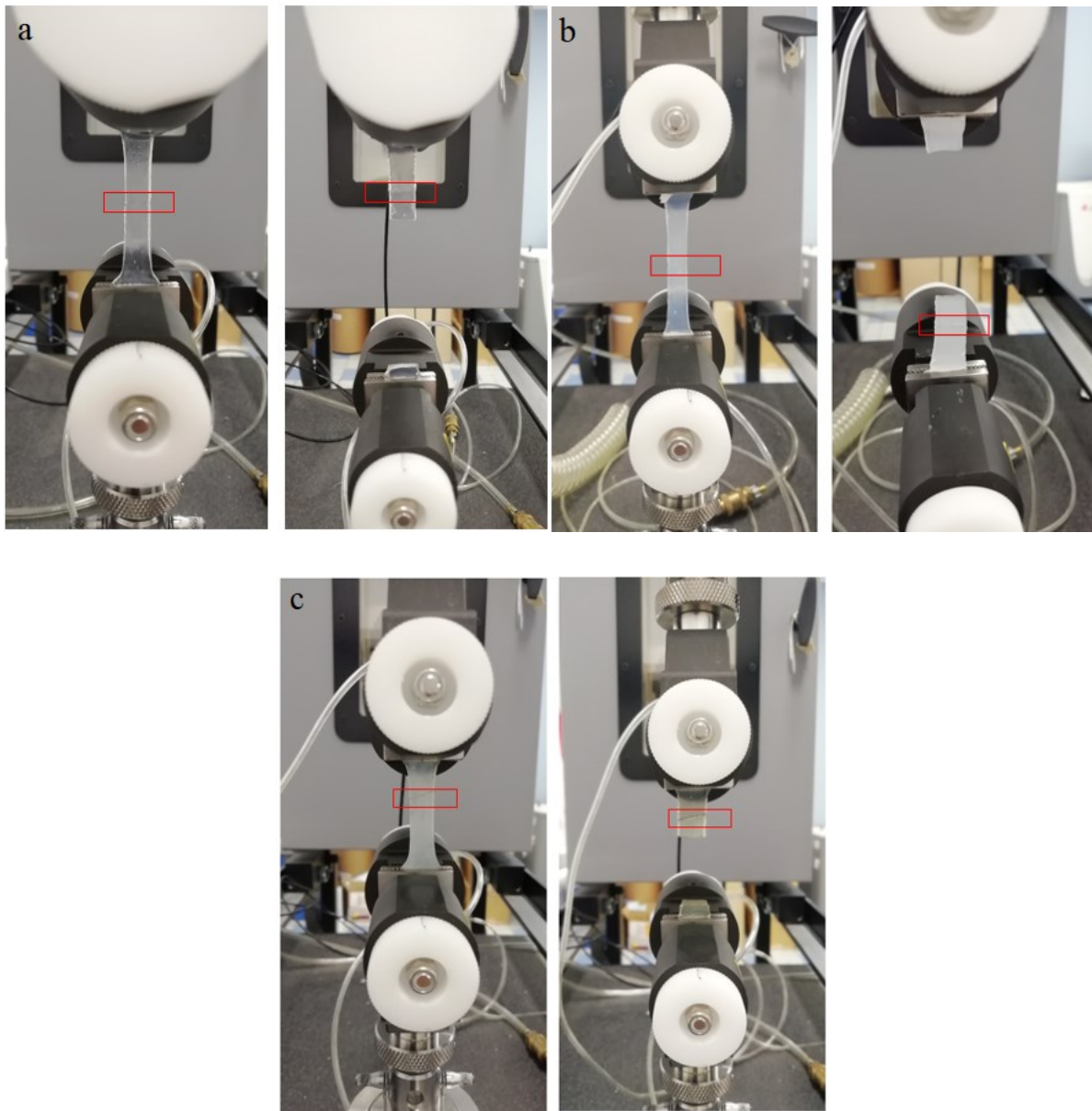
Figure 16. Tensile stress-strain measurements showing the stretching of self-healed hydrogel samples of PVA (a), PVA-CNC 1% (b) and PVA-TA 1% (c).
