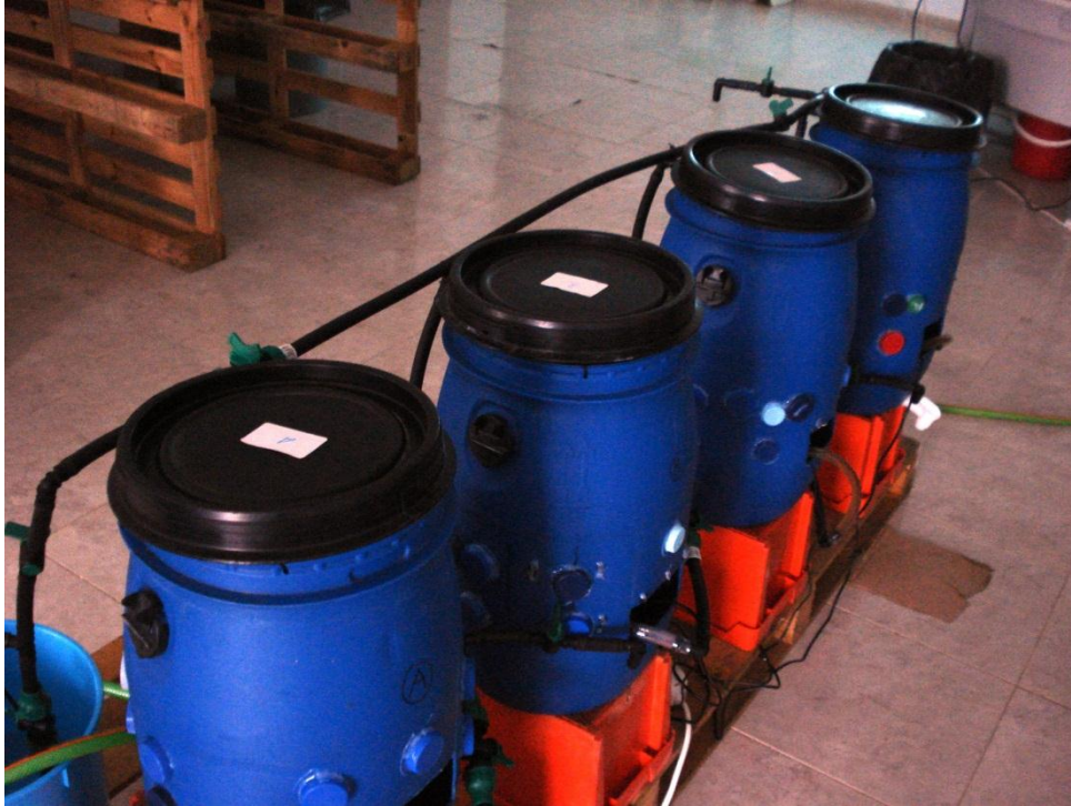
Figure A.3 – Setup of the sequential four-reactors system.
