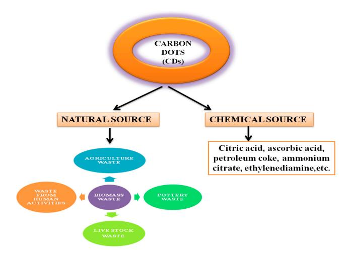
Figure 2. Natural and chemical sources of precursors used in the synthesis of CDs.
