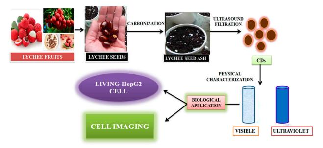
**Figure 7.** Synthesis of carbon dots from lychee seeds. The CDS were used for fluorescence imaging of living HepG2 cells, as described in [106].
