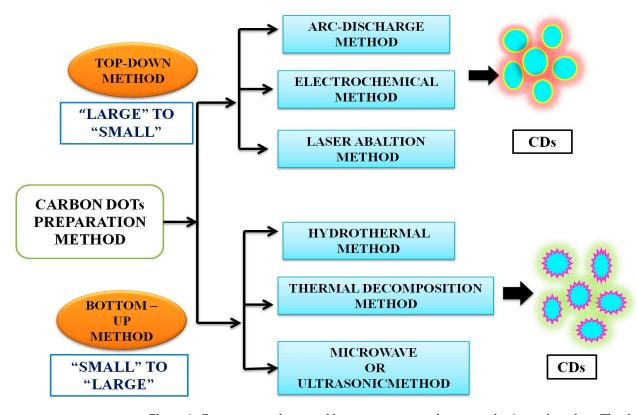
**Figure 3.** Common top-down and bottom-up approaches to synthesize carbon dots. The details of these methods are available in recent textbooks.
