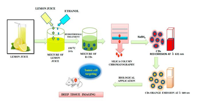
**Figure 8.** Synthesis of carbon dots from the lemon juice. The CDs were used for deep-tissue imaging, as described in [107].
