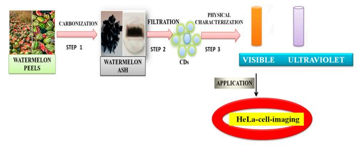
**Figure 6.** Synthesis of carbon dots from the watermelon peels. The CDs were successfully applied to HeLa cell imaging, as described in [105].
