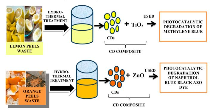
**Figure 12.** Synthesis of CDs composite from (**top**) lemon peel waste [158] and (**bottom**) orange peel waste [157] and their application for photocatalytic degradation of dyes.
