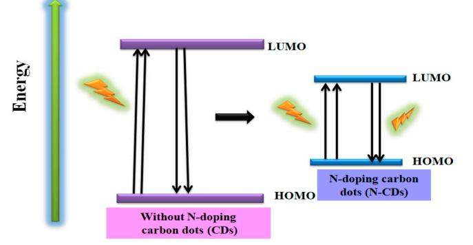
Figure 9. Energy diagram of CDs without doping and with N-doping.
