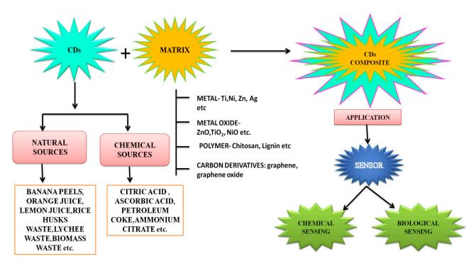
Figure 10. Overview of the synthesis of CD composites from various sources.
