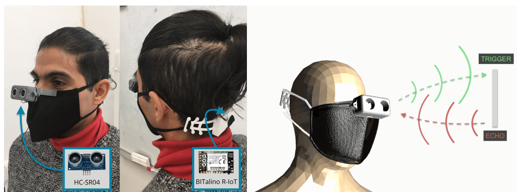
Figure 1. Proximity sensor enclosure fitted onto the face mask with trigger (output) and echo (receiver) signals.
