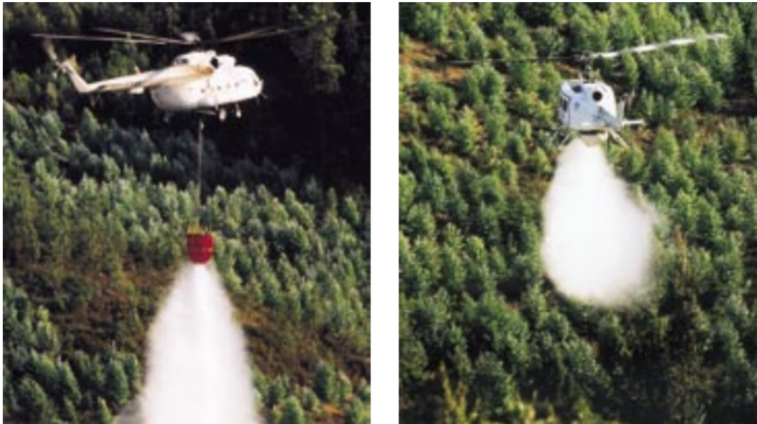
Figure 2.4: Example of helicopters used in forest firefighting. On the left, an helicopter with a bucket and, on the right, one with a water tank [3]
