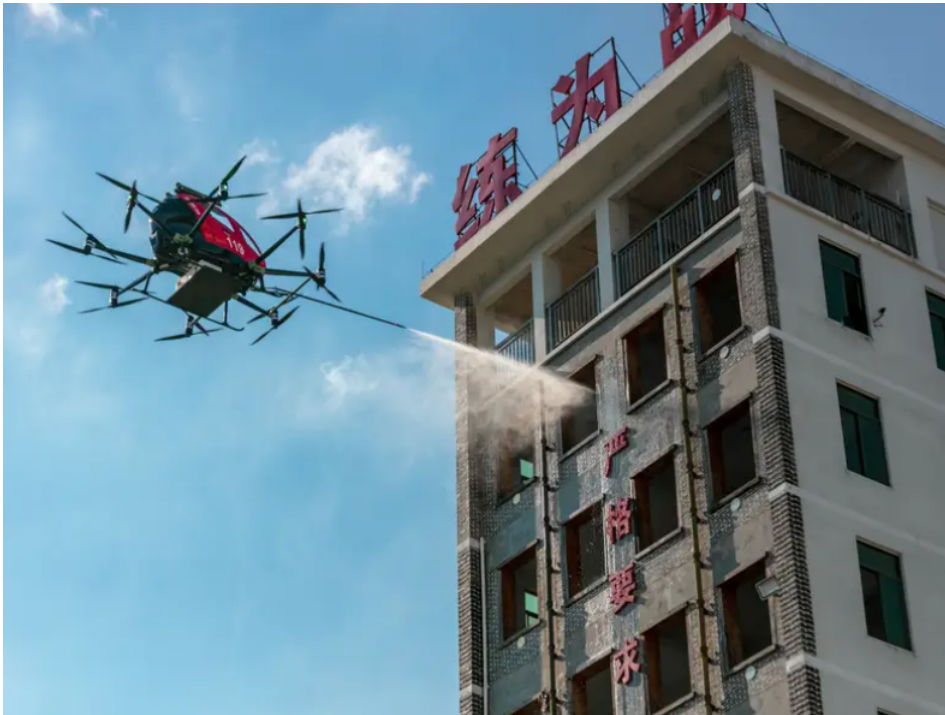
Figure 2.8: EHang's firefighting drone in action tackling a fire on a tall building [13]
