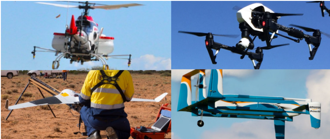
Figure 2.9: From left to right and top to bottom: Single rotor; Multi rotor; Fixed wing; Fixed wing hybrid.
