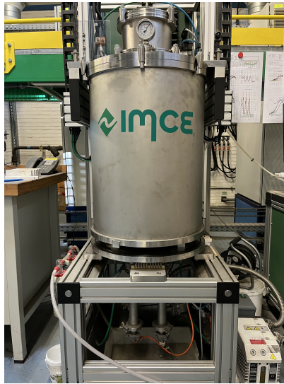
Figure 2.18: Impulse excitation technique machine available at the CRC, manufactured by IMCE NV
