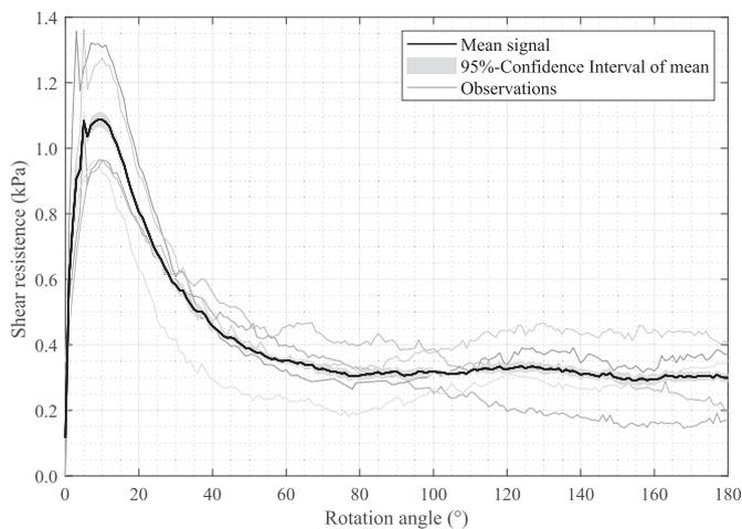
**Fig. 3.** *DiCoastar* measurements showing shear resistance curves over rotation angle acquired in undisturbed, homogenized sand samples with predefined density for a rotation angle from 0% to 180%.
