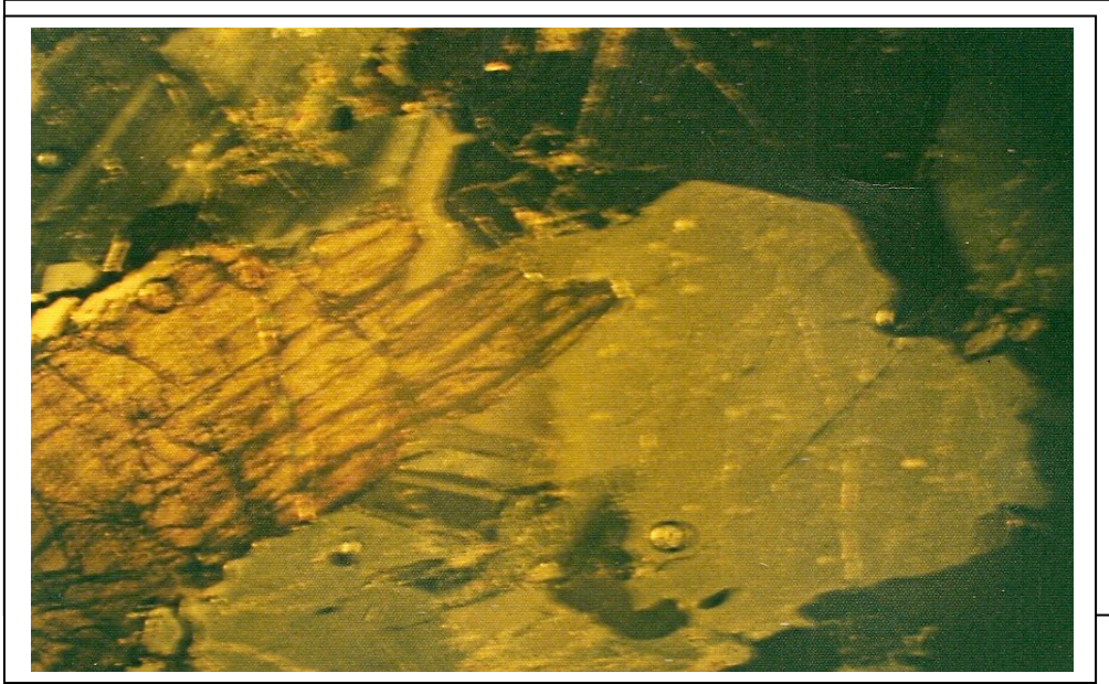
b. Feldspars are the dominant minerals showing prismatic Orthoclase and cross-hatching Microcline twinning. ( X 40)
