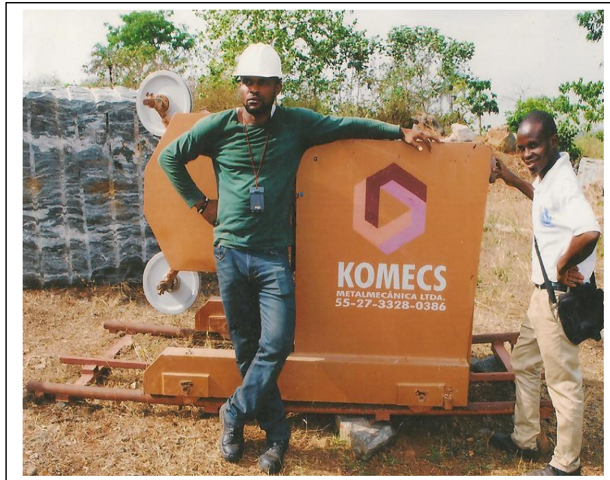
Fig.6 Dimension stone cutting machine at Octopol Quarry in Igarra
