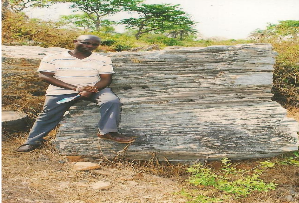
Fig.7 A block of Dimension Stone at Octopol quarry Igarra area
