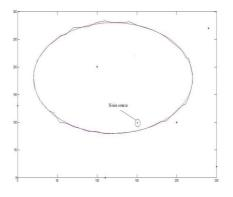
Figure8: the robot trajectory in a circular path simulation)
