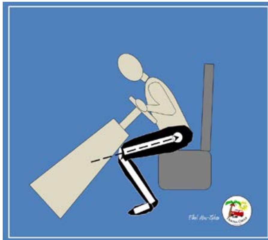
Fig 1: Males are usually taller than females. This increases their chance of having Knee-thigh-hip injuries (dashed arrow) when the knee directly hits the dashboard.
