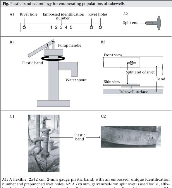
ing the band around a hand-pump tubewell, between the pump handle and the water spout; B2: Once the band is wrapped around the tubewell, the rivet is inserted through a hole at each end of the band, with the rivet's head against the tubewell surface and the two-halves of the split end splayed out and pounded flat; C1: A tubewell with plastic band still attached after 14 months; C2: Embossed identification number
