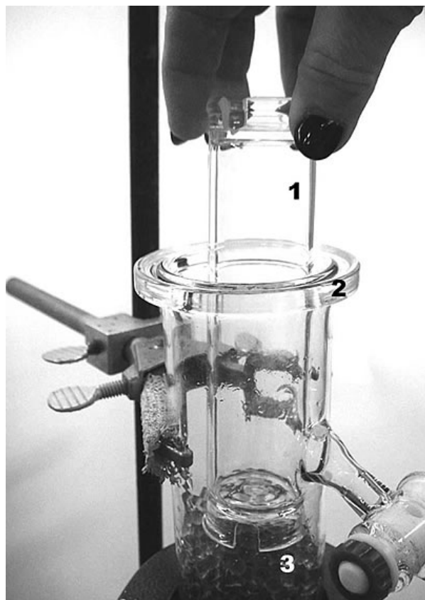
Figure 5. Insertion of a Pyrex® glass adaptor (1) into the flow-cell (2) with the top unit of the assembly removed. Alginate beads may be observed at the bottom of the assembly (3). The use of this adaptor reduces the useful volume of the assembly to approx. 30 ml. Other sizes may be used.
