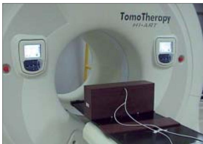
Figure 1: Hi-Art II tomotherapy machine with an ion chamber placed at 1.5 cm depth in virtual water slabs
