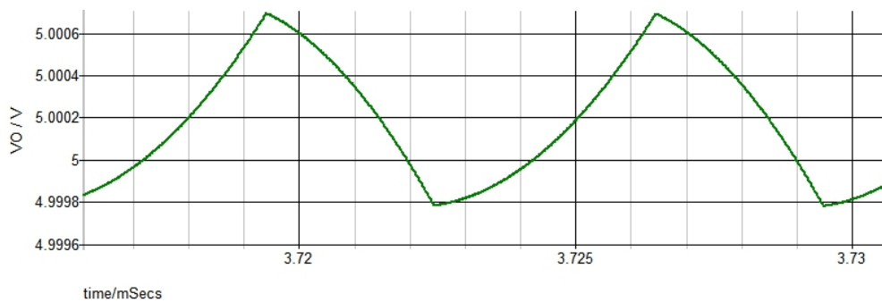
Figure 3.13 Ripple of the output voltage V_o(I_o=1.6A) in half-wave resonant.
