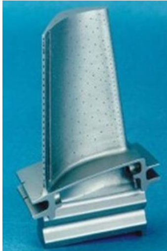
Fig. 2.18 The turbine blade with Castcool technology
