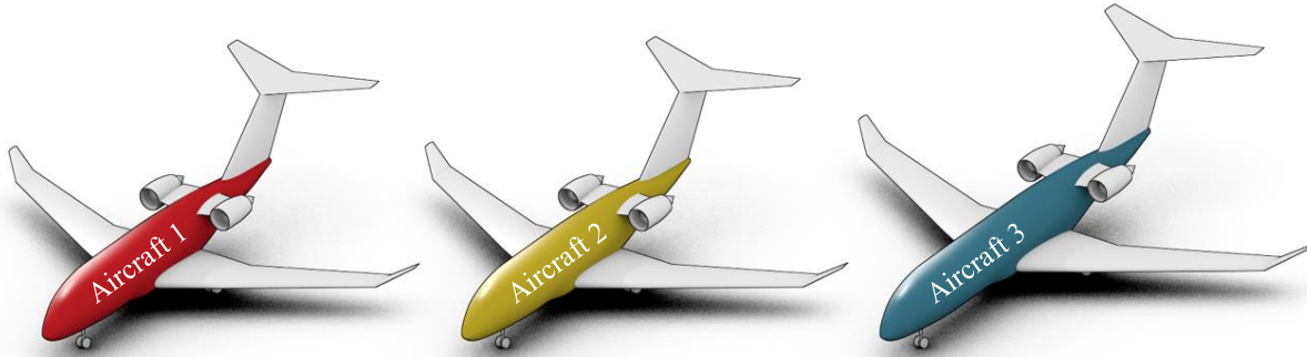
Fig. 1 Notional render of the business jet family consisting of three aircraft designed for different ranges and cabin lengths, showing aircraft with longer design ranges and larger cabins to the right, numbered 1, 2 and 3.
