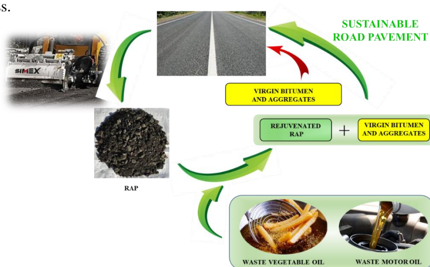
Figure 1. Schematic approach to realize a sustainable road pavement using RAP rejuvenated using waste oils.
