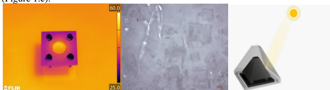
Figure 1. a) Infrared picture of photothermal coating, b) NaCl crystals obtained from the brine, c) PhAEV prototype.
