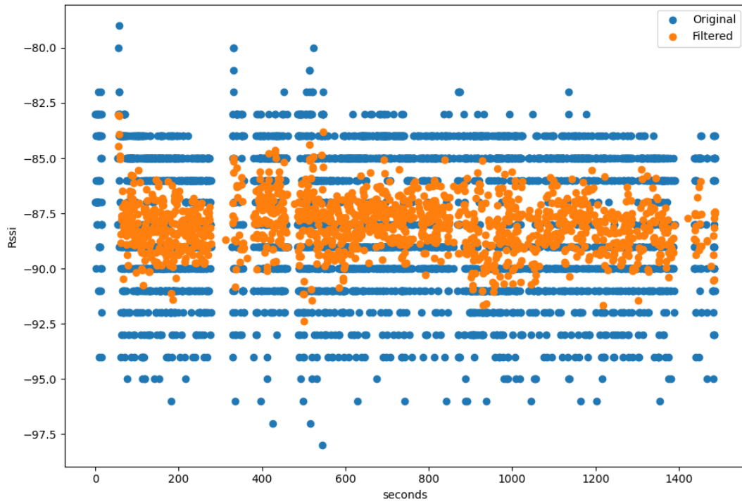
Figure 3.13: Comparison between filtered and unfiltered signal for scenario 4 at 1m
