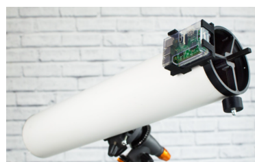
Figure 2. PiKon telescope, extracted from PiKon Website. [10]
