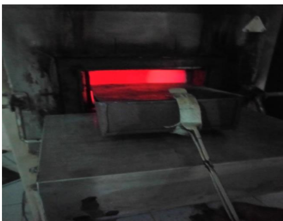
Figure 3 – Adsorbent undergoing carbonisation
