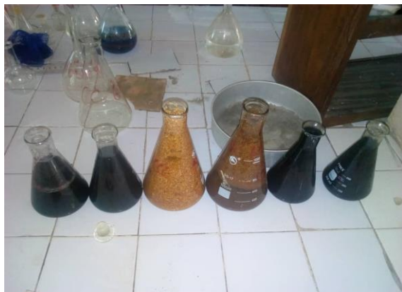
Figure 1 – Samples soaked in 0.5 M hydrochloric acid
