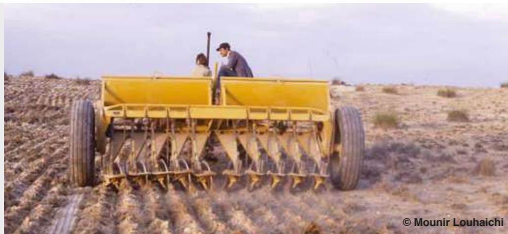
Figure 1. Mechanical seed drillers, rangeland improvement project in Kairouan, Central Tunisia
