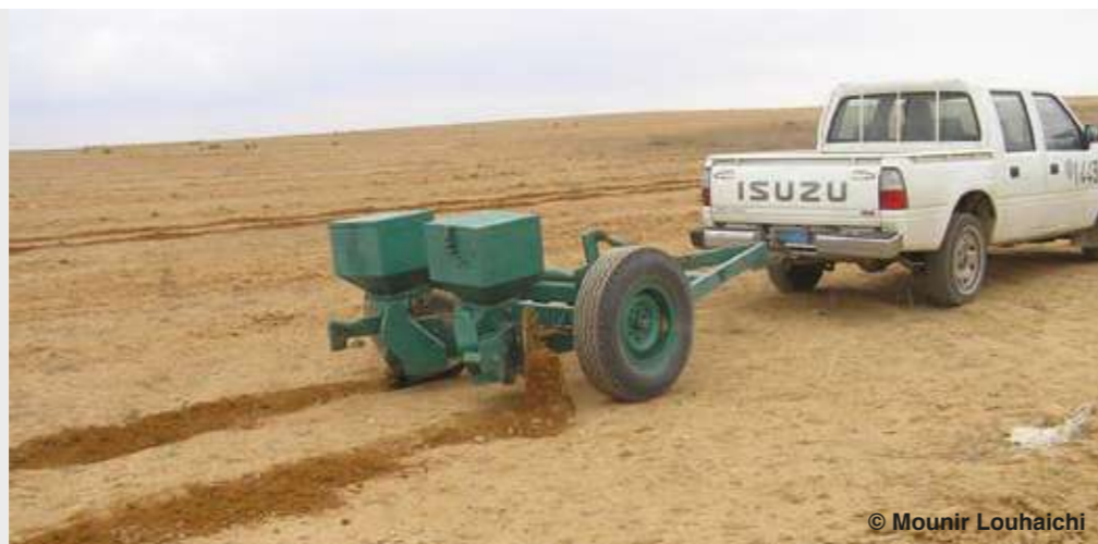
Figure 5. Mechanized direct-seeding using pitting machine, Syrian Badia
