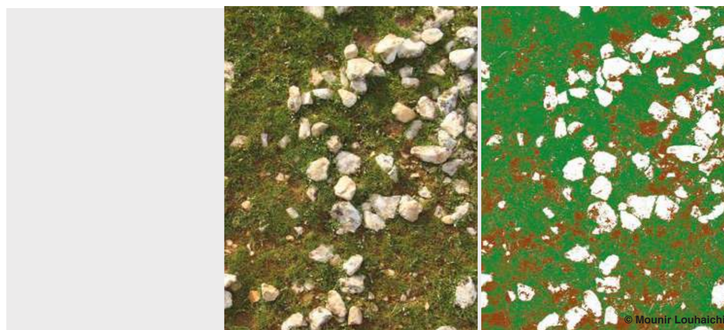
Figure 9. Original and processed images using VegMeasure software
