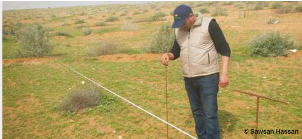
Figure 3. Vegetation cover estimation using the point intercept method
