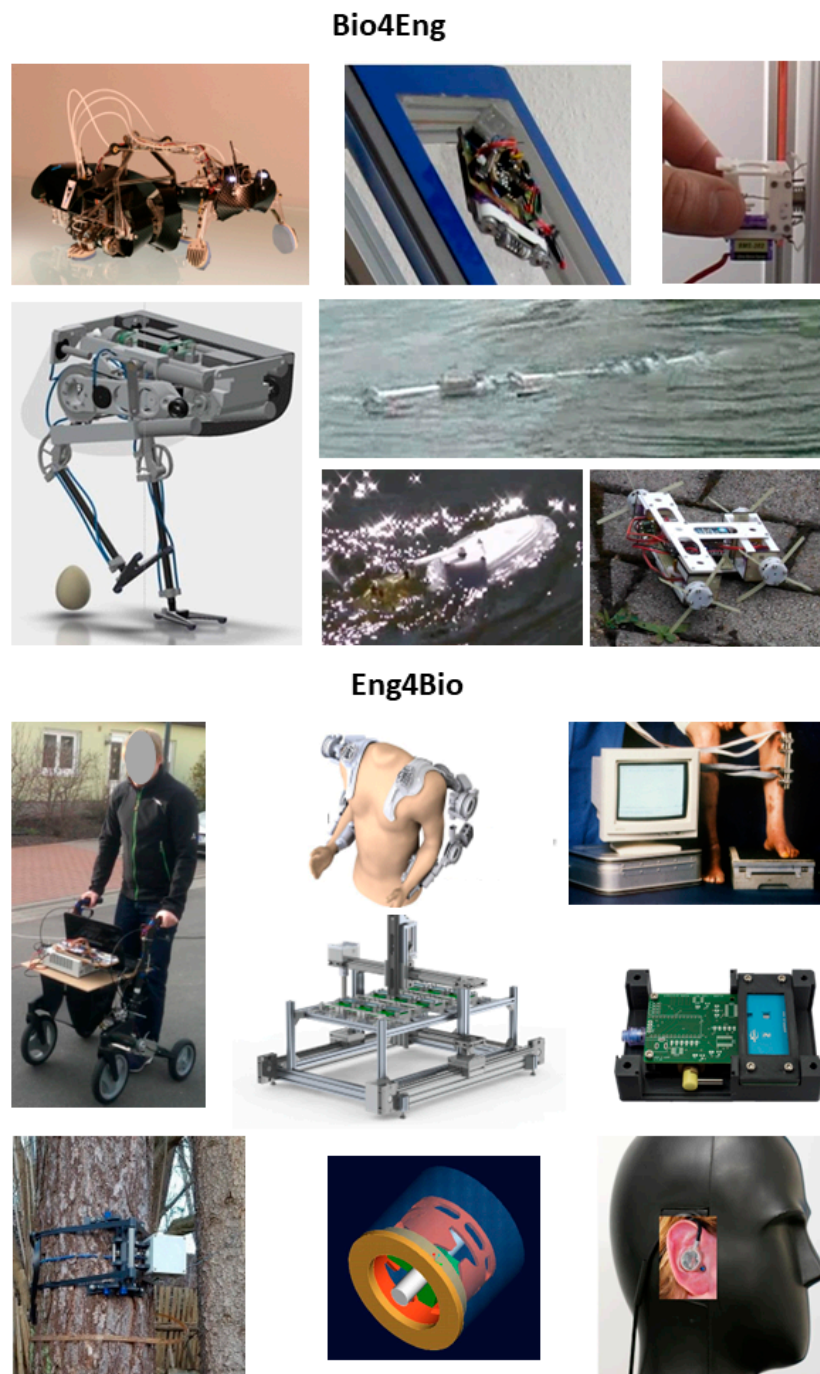
Figure 2. Examples of biomechatronic development. In reading order, please find for Bio4Eng the climbing robot RatNic (coop. Tetra GmbH Imenau, granted by the German Ministry of Education and Research BMBF) [60]; the window-cleaning robot MatBot ; the adhesive gripper TaCare ; the bird-like robot eNandu (coop. FSU Jena, Gentle Robotics); the swimming robots CSnake and Urmele ; the small wheg robot T-Whex . For Eng4Bio: the walker eRolli ; the modular exoskeleton Leviaktor (coop. FSU Jena, HS Aalen, Gottinger, BM innovations, LSK, granted by German Ministry of Education and Research BMBF), the figure is provided by Gottinger; fixateur externe instrument for measurement of fragment motions in DoF 6 (coop. RU Bochum) [61]; the system view and module of the System for Automated Cell Cultivation and Analysis (SACCA; granted by the Carl-Zeiss Stiftung); a dendrometer; a sensor for gripping forces DoF 6, 20 × 25 mm [62]; and a Personalized Miniaturized Dosimeter (PMD; granted by BGN Mannheim Erfurt) [63].
