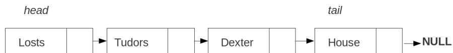
Figure 4.1: Example of a singly linked list containing my favorite series orderby preference. Each node contains a reference to the name of a TV serie and a reference to the next node (the following TV serie). The next reference of the last node (tail) links to null .
