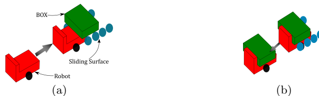
Fig. 1: (a) Entry movement to accommodate the robot under the rack, (b) Exit movement to load the product on the robot.
