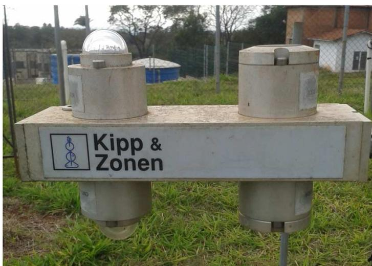
Figura 4 - Saldoradiômetro CNRI Net Radiometer.
