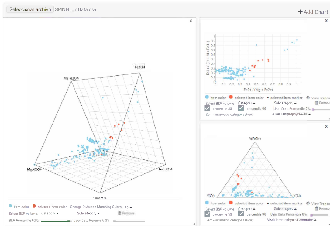
Figure 9: Screenshot of an analysis session in which geologists interact with different views of the data: the spinel prism (left), and the triangular (bottom right) and lateral projection (upper right). A brushing is activated (red points) and highlighted in all coordinated views [28].
