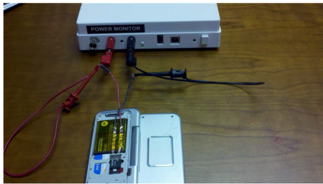
Fig. 4. Power Monitor setup
