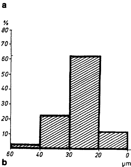
Fig. 5. Granulometric analysis of Sample B4. (a) Particle-size distribution; (b) frequency distribution of particles as a function of size
