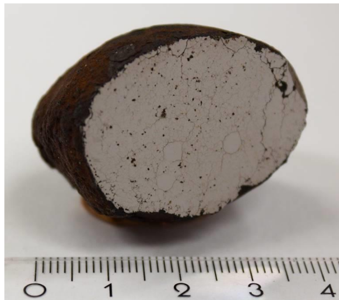
Figure 1. The endcut of Lieksa-4 showing its reflective material and the internal structure. The meteorite consists of small ( \leq 0.5 mm), round granules with a few larger ( \sim 3.0 mm) granules present as well. The outer layer is covered in a thick ( \sim 1 mm) layer of rust, suggesting that Lieksa-4 has been on the ground for an extended period.
