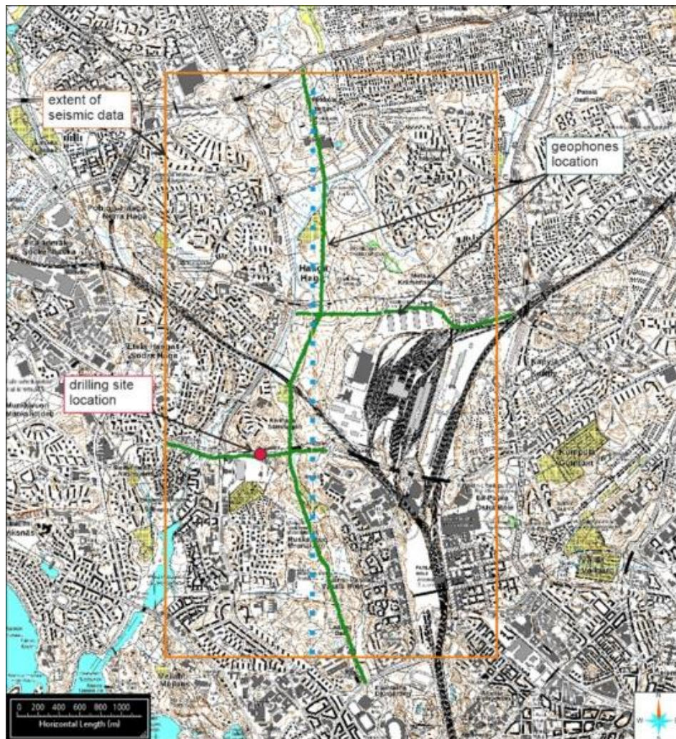
Figure 1. Location of Keskuspuisto semi-3D seismic survey overlaid on the Helsinki city map (map source: National Land Survey of Finland). The green lines mark the locations of geophones; the orange rectangle is the extent of the seismic data; the red dot points to the Ruskeasuo drilling site. The dotted blue line marks the seismic cross-section shown in Figure 2.
