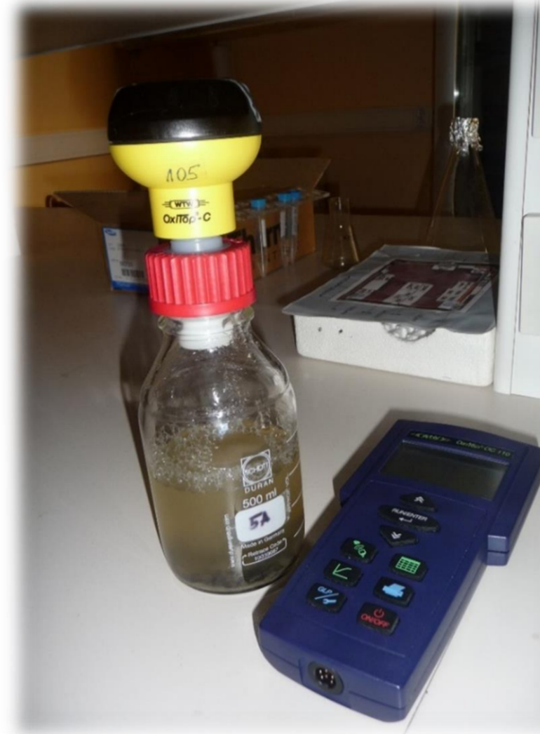
Figure 2. Pressure increase measurement with OxiTop system (WTW, Germany).
