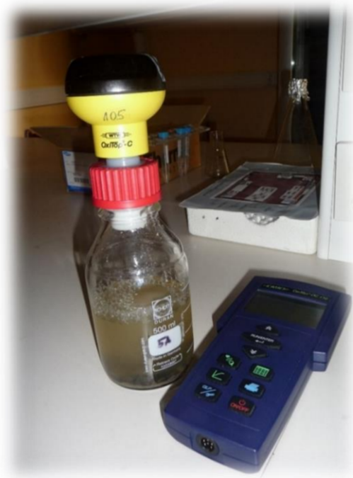
Figure 1. Pressure increase measurement with OxiTop system (WTW, Germany).
