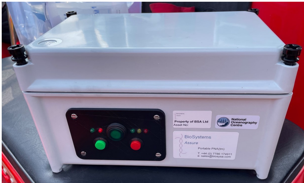
Figure 12: A photograph of the portable DNA analysis system prototype outer shell, which was used to demonstrate the concept of in situ DNA/qPCR analysis. The system was developed by collaboration between the National Oceanography Centre and BioSysA Ltd.
