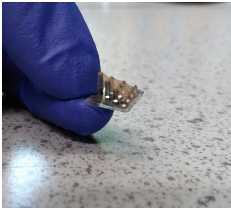
Figure 9. A prototype of the device including electrospun PVDF nanofibers mimicking the tip-link behavior on top and PDMS pillars substrate.
