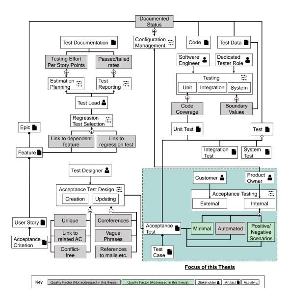
Figure 9.3: Activity-Based Quality Model for Agile Test Artifacts. In This Thesis, We Propose an Approach Capable of Automatically Creating Acceptance Tests in Compliance With the Two Quality Factors **Positive and Negative Scenarios** and **Minimal**. The Focus of Our Thesis Is Highlighted by a The Focus of Our Thesis Is Highlighted by a Green Frame.
