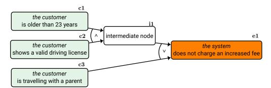
(a) Cause-Effect-Graph. Antecedents Are Represented as Cause Nodes (Highlighted in Green). Consequents Are Illustrated by Effect Nodes (Highlighted in Orange).
