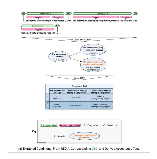
**Figure 10.3:** Overview of the Conditionals Extracted by CiRA in Fine-Grained Form, the Generated *Cause-Effect-Graphs*, and the Derived Acceptance Tests per Requirement Defined in the THEMAS Specification.
