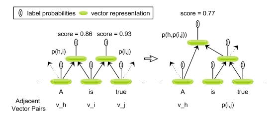
Figure 2.4: Bottom-Up Approach of an RNTN for the Prediction of a Binary Parse Tree, Based on [128].
