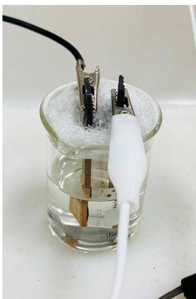
Figure 1.7 Electrochemical cell with two electrodes (EMD vs. AC).
