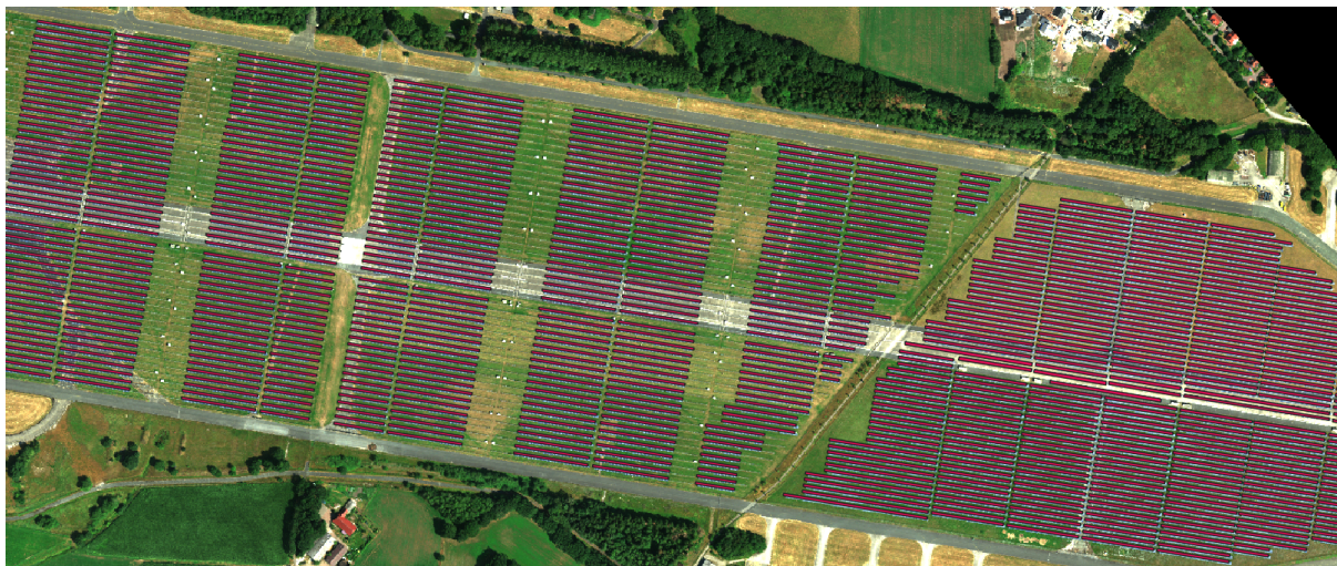
Figure 1: Detail of ground truth in vectorial format for solar panels (red), overlaid on HySpex true color composite.
