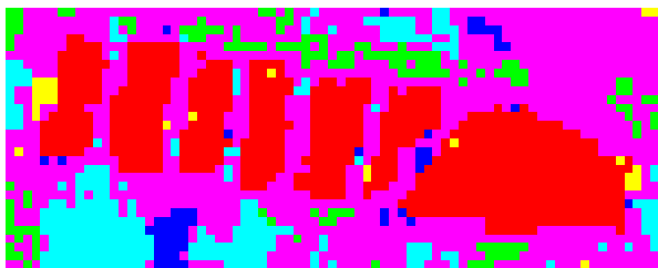
Figure 5: DESIS Maximum Likelihood results. Solar panels class is reported in red.
