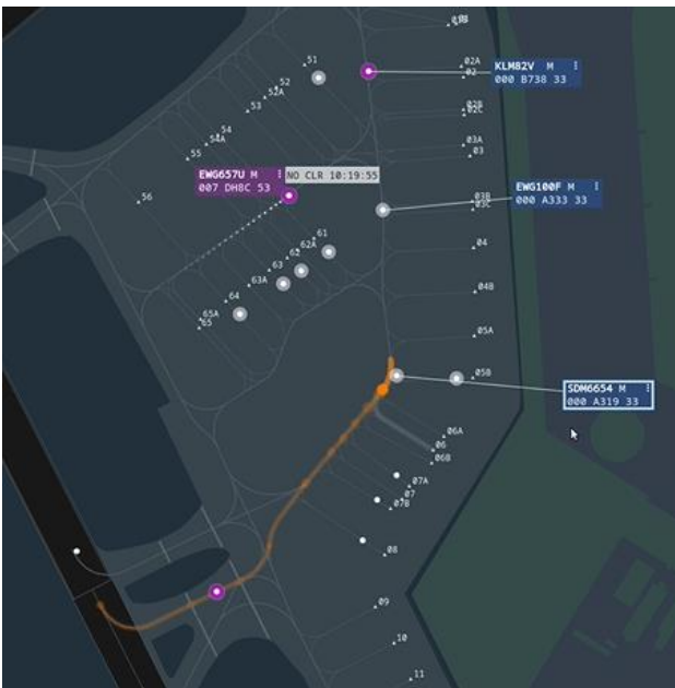
FIGURE 1. Cut-out of the traffic situation display showing 1) an alert at the label of the flight EWG657U: 2) a trajectory for flight SDM6654 and 3) an advisory marker (pink ring) at KLM82V, showing that the taxi clearance is recommended now for this flight.
