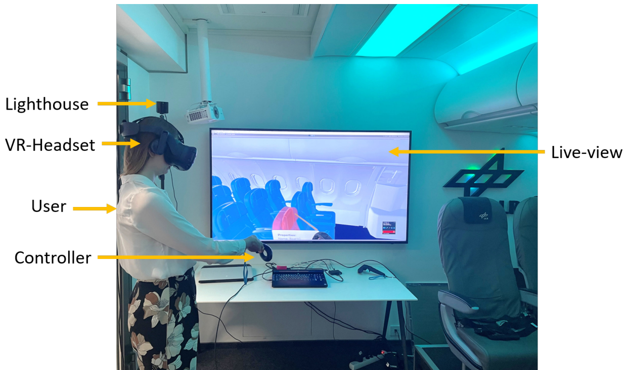
Figure 5 – Setup of the virtual reality laboratory for testing and assessing cabin concepts.
