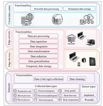
FIGURE 1. Edge-assisted smart healthcare functionality flow.
