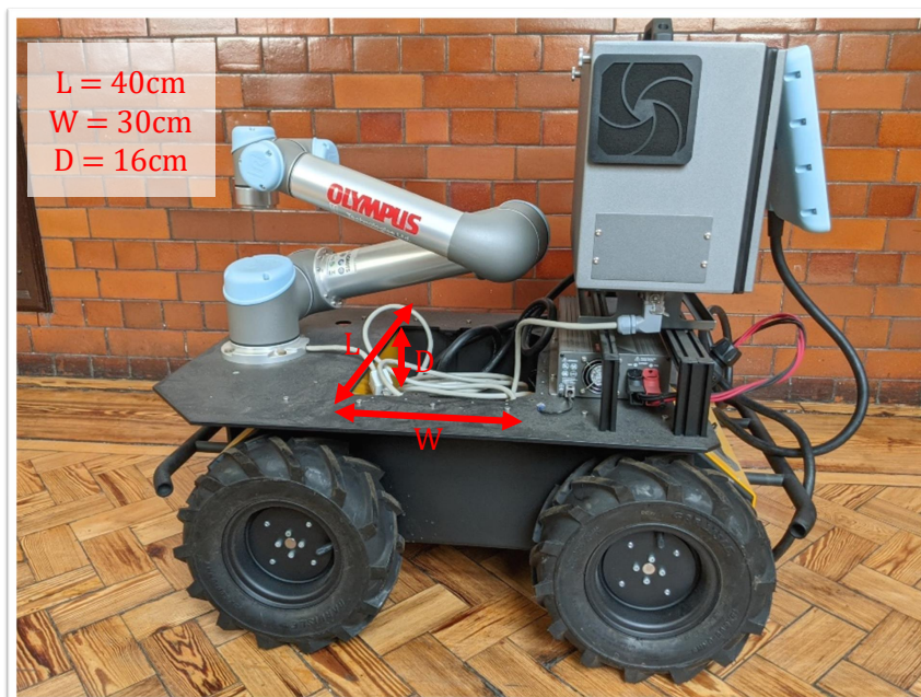
Figure 6.2: An image of the Clearpath Husky robot fitted with an arm. Dimensions for the operational area where equipment may be mounted are highlighted in red.
