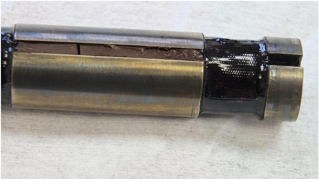
Figure 154 TIRPI post testing thermal inspection discolouration of hot region
