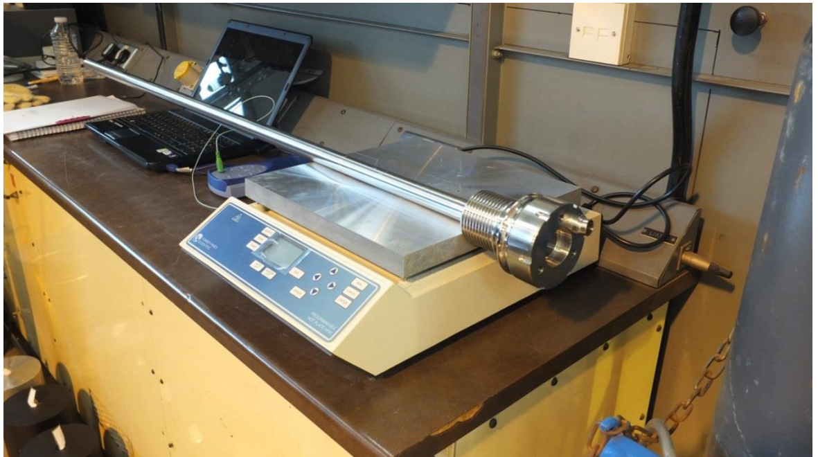
Figure 118 Probe tube hot plate testing setup
