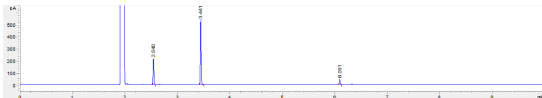
Figure 144: GC-FID chromatogram for the biotransformation of the reductive amination between cyclopentanone and aniline
