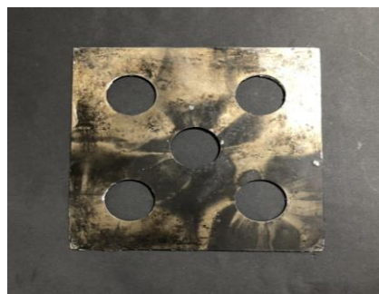
Figure 3.24: Compression mould for rheology samples with a thickness of 1.00 \pm 0.05 mm and a diameter of 25.00 \pm 0.05 mm
