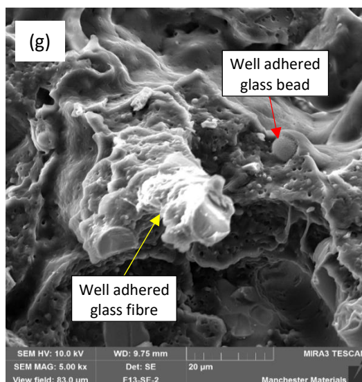
Figure 5.21: The micrographs of the fracture surfaces of Izod sample at 5000x of PP hybrid composites with 30 wt% of glass fibre and different glass bead contents (a) 1 wt% (b) 5 wt% (c) 7.5 wt% (d) 10 wt% (e) 15 wt% (f) 20 wt% (g) PP hybrid composites with glass bead 10 wt% and glass fibre 40 wt% at 5000x
