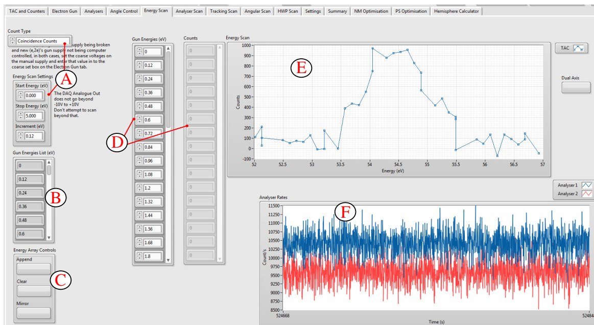
Figure 5.24: A screenshot of the gun energy scan tab in the main control program. Label A shows the scan settings: the count type for the scan and the gun energies to add to the scan. Label B shows the list of gun energies to add to the scan and C shows buttons to append to, clear, or mirror the gun energies in this list to the scan. Label D shows the gun energies to scan and the counts measured at each step. Label E shows a graph of the counts with respect to gun energy and F shows the current analyser rates.
