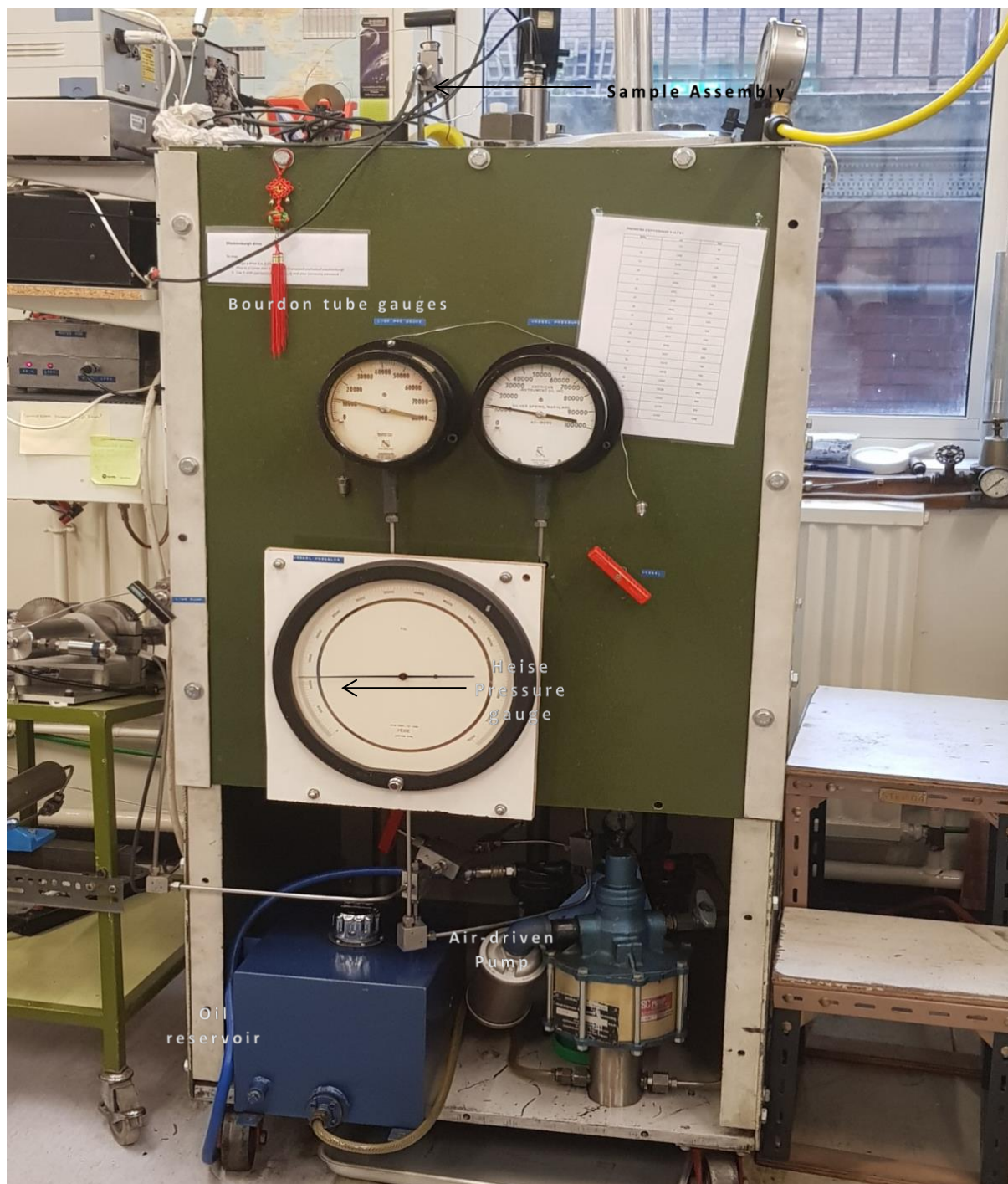
Figure 4.17 The Green Rig apparatus used for the acoustic wave velocity measurements. The green panels are the steel plates that provide safety screening for the user. The left-hand side has the electrical system used for control functions and for monitoring the data. The vessel uses oil as a confining medium while argon gas is used as pore fluid. The pore pressure volumometer for argon is mounted behind the apparatus and is identical to the pore volumometer dedicated for use with water that can be seen to the left of the Heise pressure gauge.
