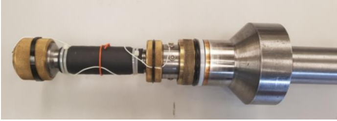
Figure 4.19 A sample assembly for acoustic velocity experiments, with the 25 mm diameter specimen inside the (black) heat-shrink rubber tubing, between the two transducer housings. At the right hand end is the closure plug that seals the top end of the pressure vessel.
