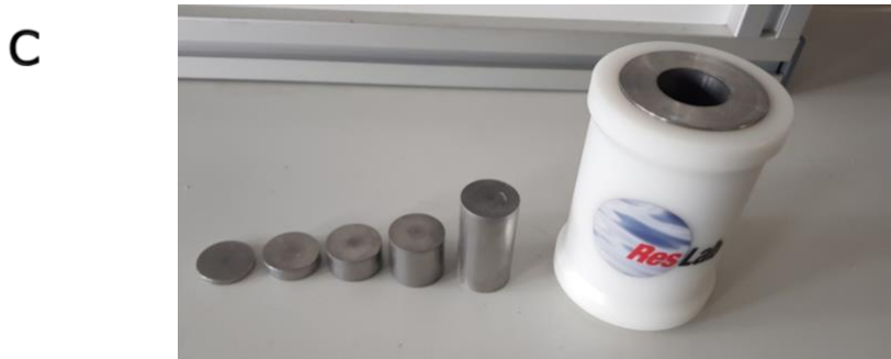
Figure 3.23 A) External photographic view of the Res Lab Porosimeter B) A schematic diagram showing the layout of the Porosimeter, with a representation of a porous rock cylinder inside volume V_2 C) Specimen vessel (volume V_2 ) and calibration disc set provided with the Porosimeter.
