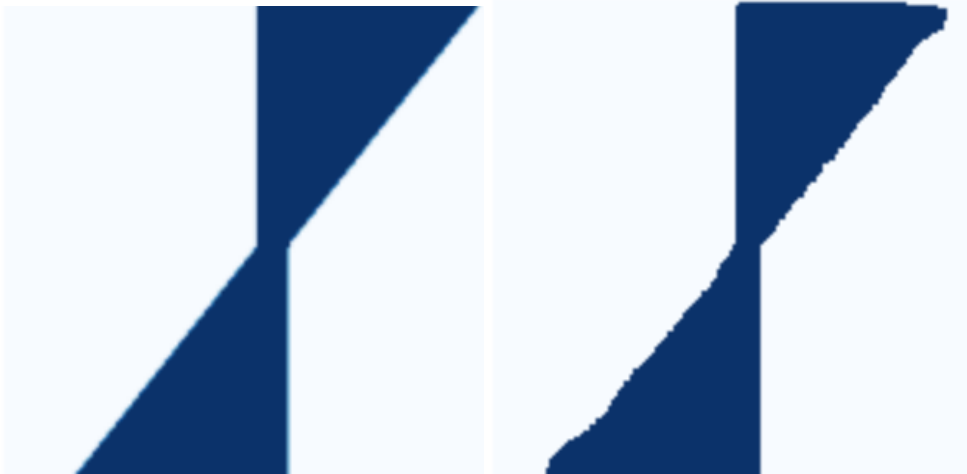
Figure 8.9 – Illustration of the segmentation mask. The training target for the mask branch is illustrated in the left panel. This stage takes the detections (refined bounding boxes and class IDs) from the previous layer and runs the mask head to generate segmentation masks for every instance. The predicted mask is shown in the right panel.
