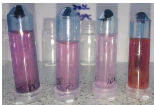
Figure 3.15: Left to right: Synperonic F38 PDPPF4 emulsions (entry 3.25) precipitated in MeOH, EtOH, iPrOH and n-BuOH. Polymer pellets were observed in all 1.5 mL centrifuge tubes.
