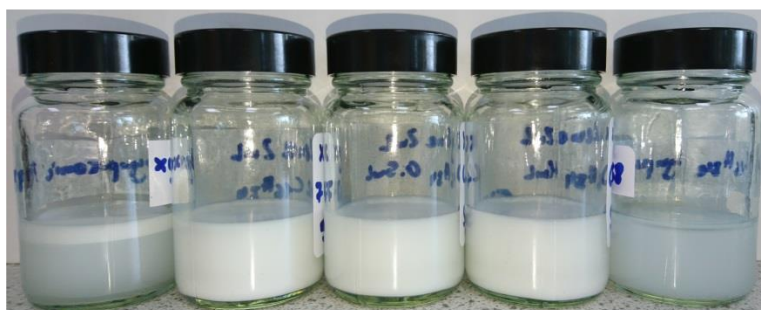
Figure 3.17: Blank samples of Synperonic F38 emulsions with different hexadecane concentrations with increasing hexadecane content from left to right according to table 3.11.
